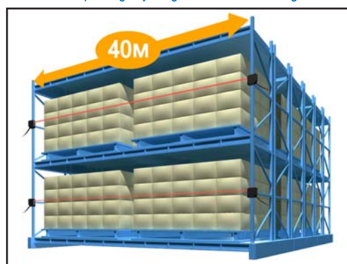
Detection of packages jutting out from their storage location
